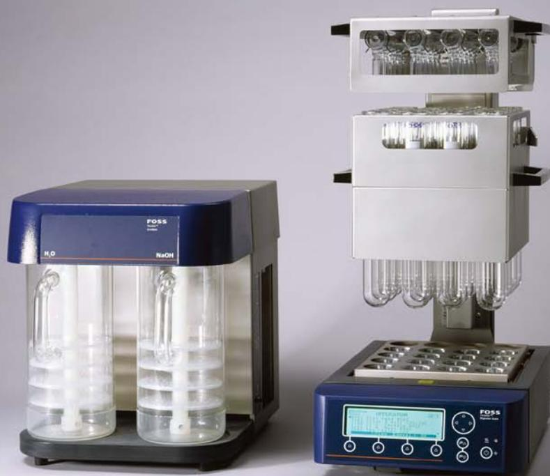
*Tecator™ Digestion Unit Auto Lift 20 together with the Scrubber, for fully unattended operation.*
