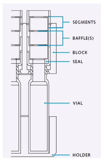
The toolkit is entirely modular, enabling the researcher to create their own baffle configurations to achieve the desired evaporation time profile for a set of solvents. Increasing the evaporation temperature can speed up the evaporation rate, however, care must be taken not to exceed the boiling point of the most volatile solvent present.
